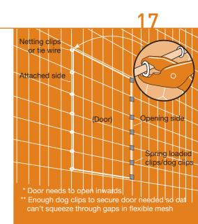
Figure 8: Design and construction of door
