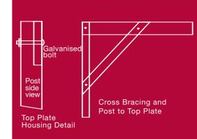
Figure 3: Top plate housing
