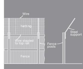
Figure 3: Completed steel support with netting
