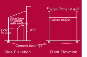
Figure 7: Tubular steel enclosure
